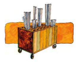
cart identification number and bin location is displayed for each mainframe or sash component, allowing each window component to be easily pulled from its designated cart bin location and loaded into the machine.
