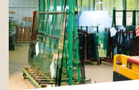
Optimization of flat glass cutting produces higher yields when a wide variety of sizes are considered. Yet, the larger the mix at cutting, the greater the loss in production control because of sorting.
